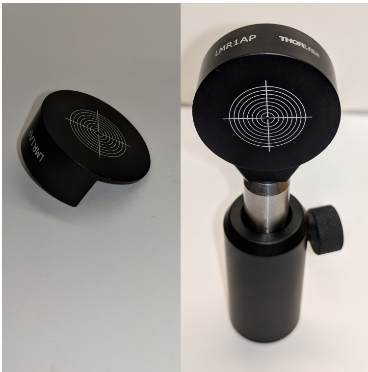
FIGURE 10.14 A target can be hung on a one-inch circular optic for alignment.
