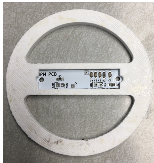
FIGURE 21.14 SiPM PCB back side. SiPM PCB circuit elements are soldered on the back.
