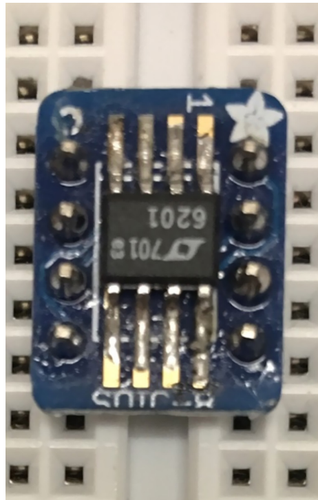
FIGURE 21.19 An LT6201 dual op amp soldered to a surface mount IC breakout board.
