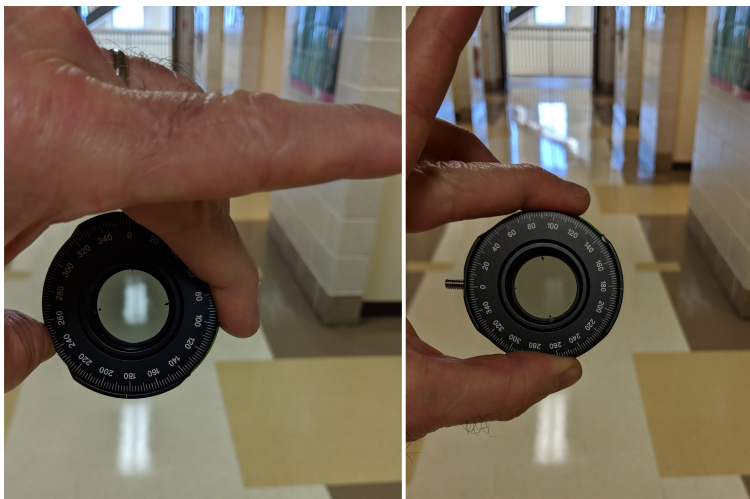
FIGURE 10.9 Roughly checking polarization axis. Left: the light from the overhead lights down the hall is reflected off the floor. The reflected light is mostly horizontally polarized. The transmission axis of the polarizer is horizontal, so the light gets through. Right: the transmission axis is vertical, so the light is blocked.
