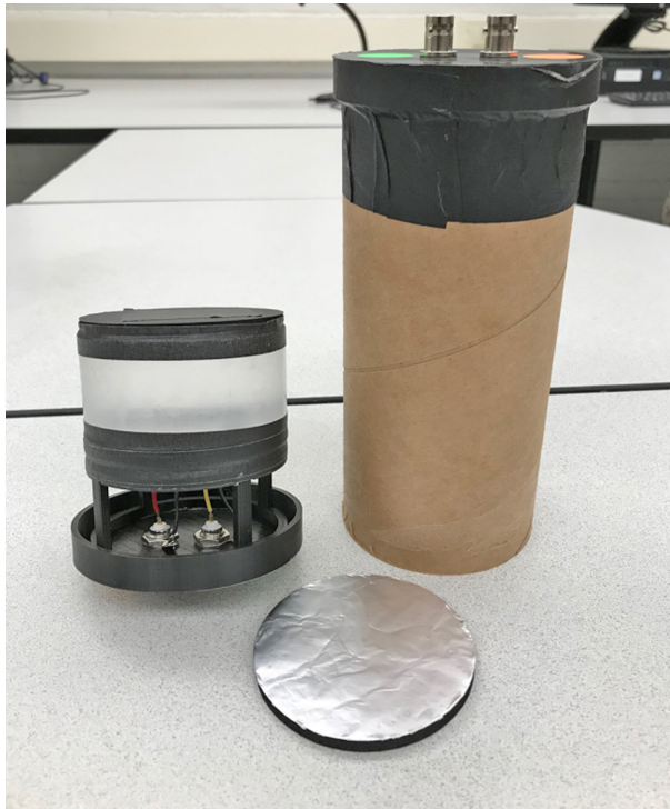
FIGURE 21.16 At the center front is an example of a disk with aluminum foil attached. On the left is a completed detector assembly, and on the right is a detector assembly installed in a tube.
