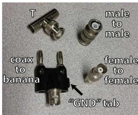
FIGURE 6.54 Four types of coax adapters. For the coax-to-banana, the banana on the “GND” tab side is connected to the outer coax connector, which is often connected to ground.
