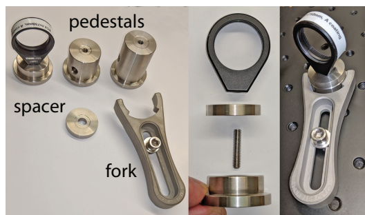
FIGURE 10.5 Left: pedestal system. Middle: assembly including spacer ring; note long setscrew. Right: fully assembled with spacer ring.
