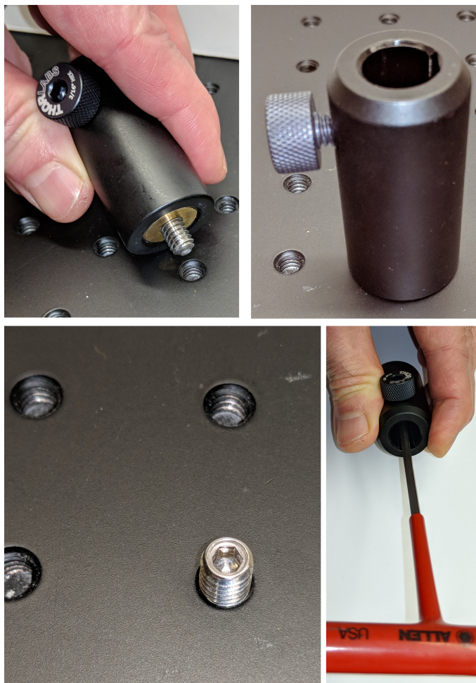
FIGURE 10.2 Top images: screwing a postholder into the optical table. Bottom row: After disassembly, if the screw was put with the Allen head up (toward the post holder), it can be easily removed whether it winds up in the table or in the postholder.
